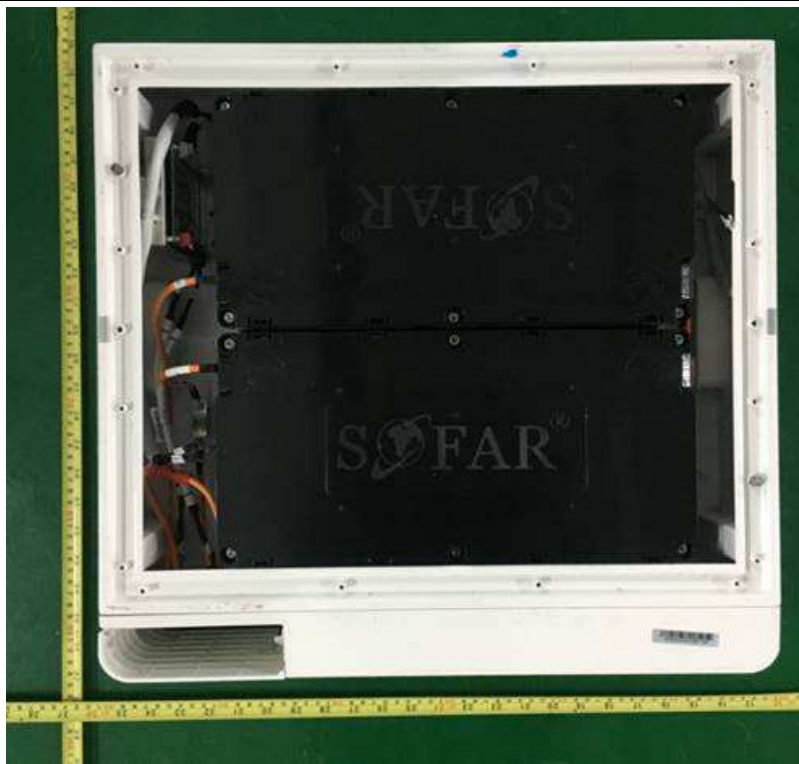
Internal view-1 of battery expansion modules
